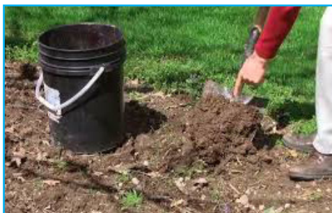
When gathering soils for testing, Take samples, when the soil is not too wet, from multiple spots in your field and mix them together.
