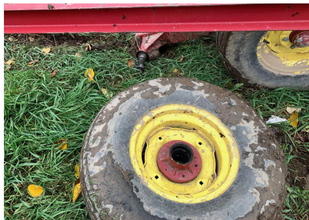
An image of the broken tire and rim.
